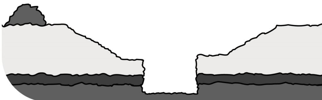
Figure 11 Combination of benching and battering controls
