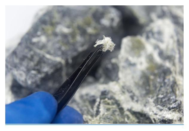
Chrysotile asbestos (white) is the most common type of asbestos used in Australia.
