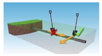
Another safe method of potholing is vacuum excavation which is a fast and usually non-destructive way to locate and expose underground utilities services. It must be noted that water jetting at some high pressures can damage cables and pipe coatings.
