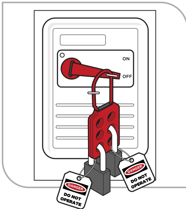
Figure 5: Locking off methods incorporating danger tags – danger tagged locking off hasp
