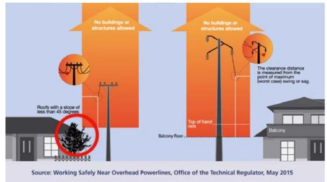
When positioning a building on site, you should allow for the width of any scaffold you may need to erect. This is to ensure the scaffold can be positioned in a way that legal safe clearance distances are met.
