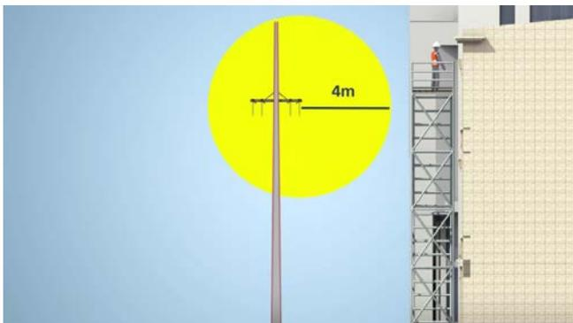
The minimum safe clearance distances are measured from the power line to the final position of the scaffold.
