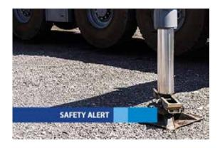
Crush risk when operating stabilisers on truck mounted cranes
